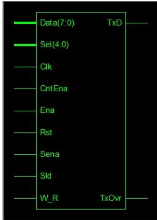
Figure.9 RTL schematic of ZigBee transmitter
